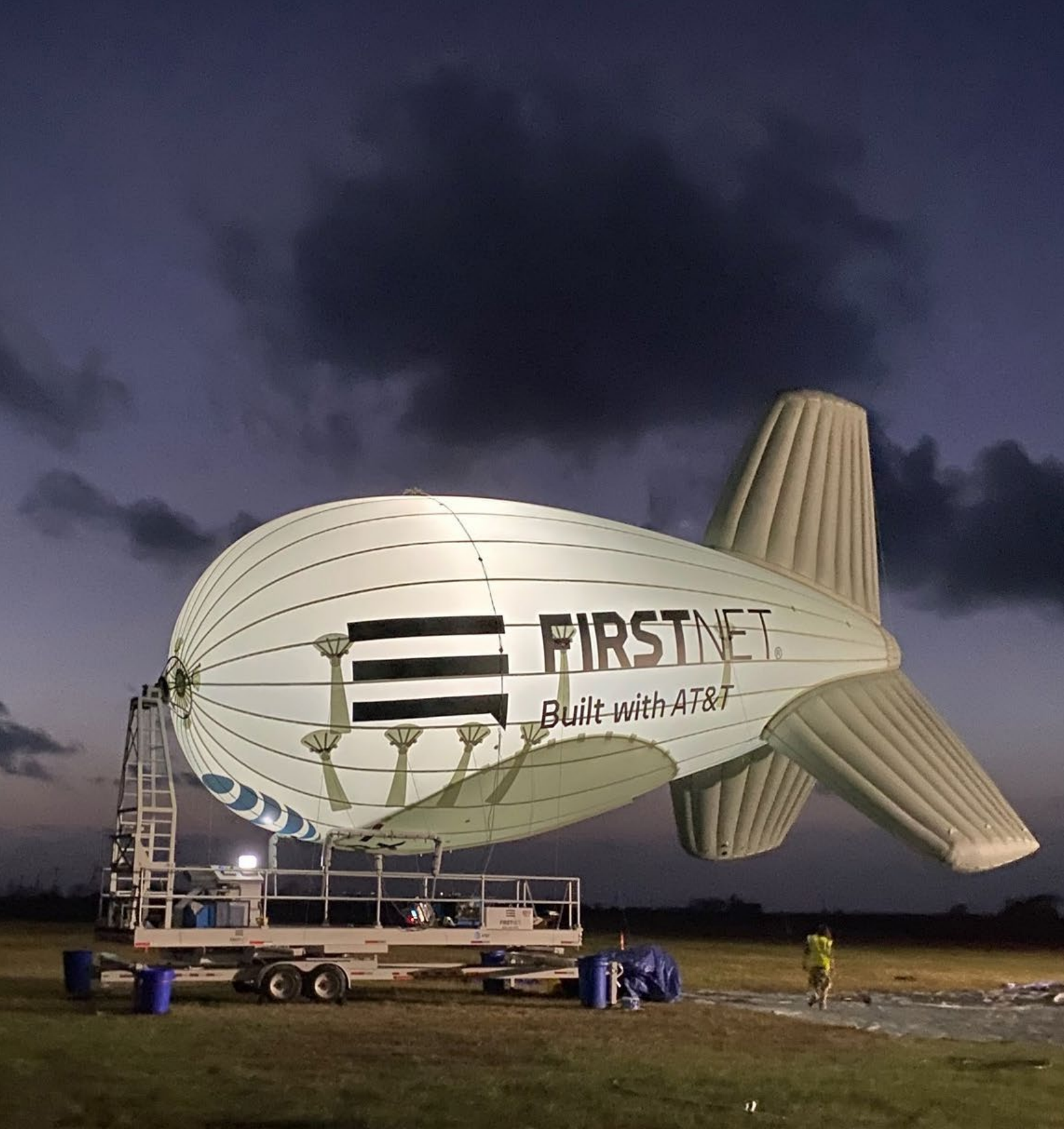
FirstNet One—an approximately 55-foot aerostat—deployed to Cameron Parish, Louisiana, in the aftermath of Hurricane Laura to support first responders by extending coverage to a wider area.
