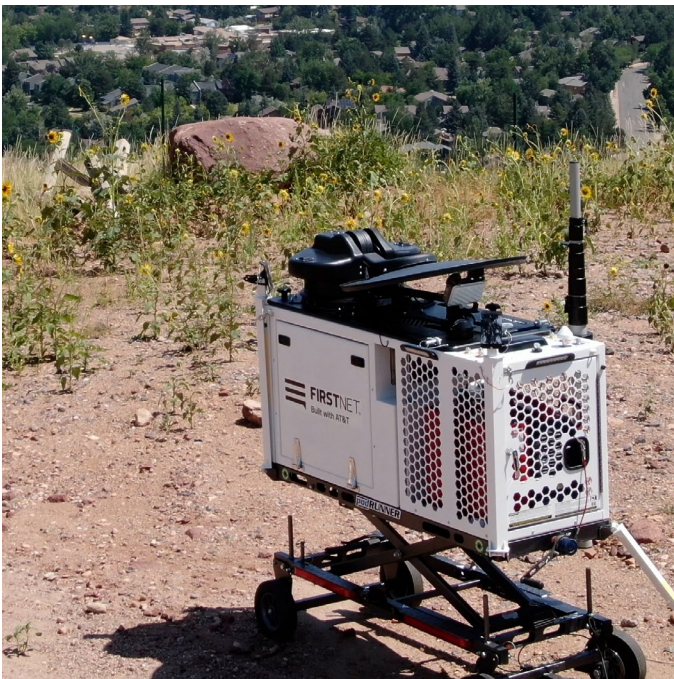
A FirstNet Compact Rapid Deployable in the field in Colorado.
